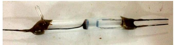
Figure 7. Produced X-ray tube
