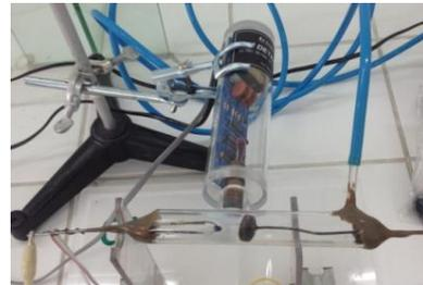
Figure 12. Geiger-Muller counter and X-ray tube
