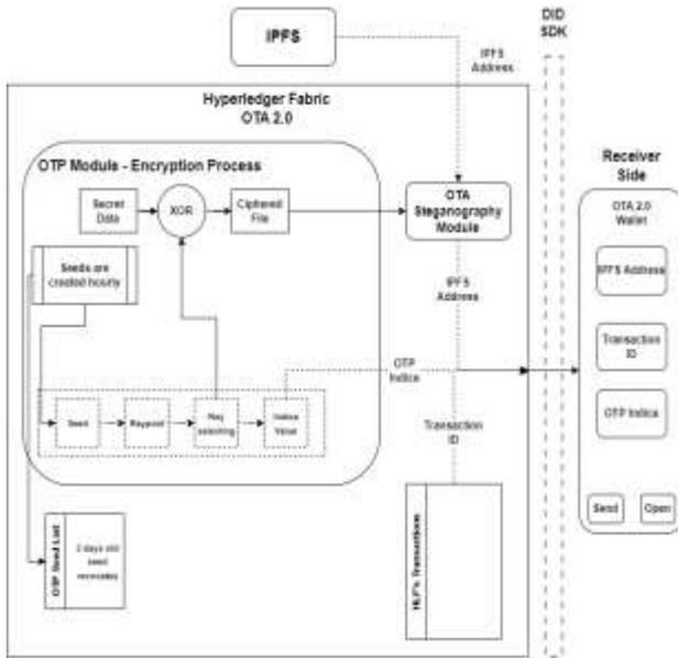
Figure 9. Structure of encryption process.
