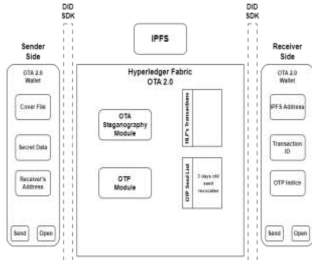
Figure 8. Structure of OTA(2.0) algorithm.
