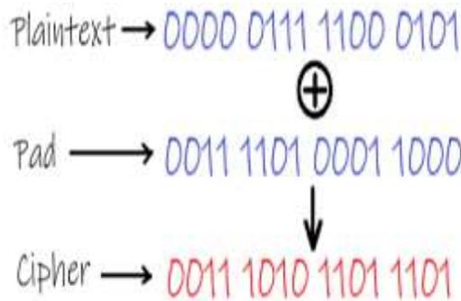
Figure 5. Steps of One-Time-Pad symmetric encryption.
