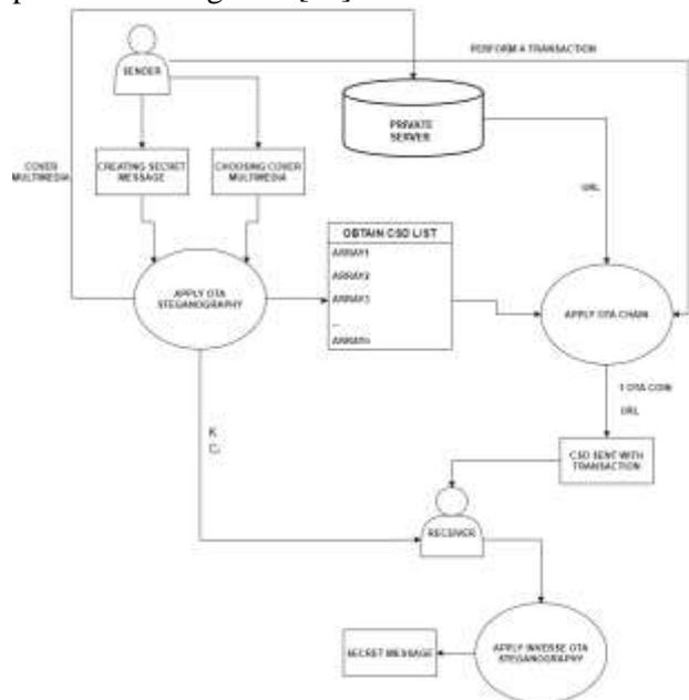
Figure 7. Structure of OTA(1.0) algorithm [20].
