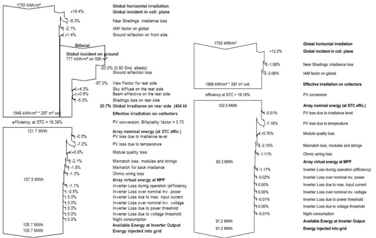
Figure 9. Loss Diagrams of Bifacial (left) PV installed on White Ground and monofacial (right) PV Panels
